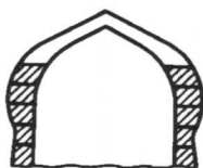
Fig. 96. Thrustless selfbalanced dome
