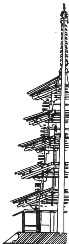
Fig. 108. The Japanese pagoda with flexible core
