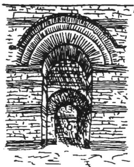
Fig. 67. Heavy-duty arch and reinforcing a stone wall with brick tiers
