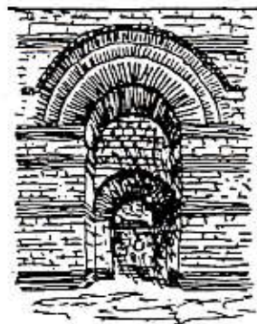
Fig. 36. Superreliable Arch and Reinforcing Stone Masonry with Brick Courses
