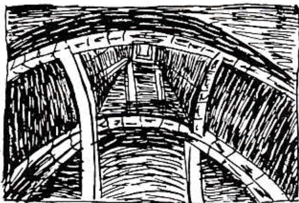
Fig. 45. Arched Skeleton for Supporting Dome
