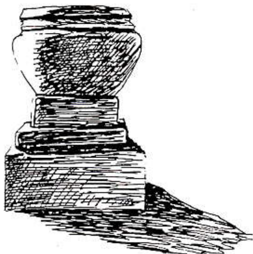
Fig. 62. Stone Base of Wooden Column
