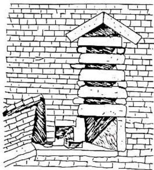
Fig. 15. Unloading System of Burial Chamber and Galleries of Great Pyramid of Cheops
