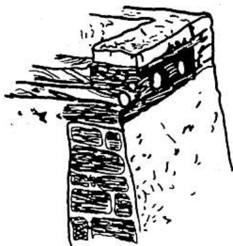
Fig. 84. Earthquake Resistant Joint Between Roof and Wall in Tibetan Dwellings
